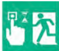
Signage for system with time delay
